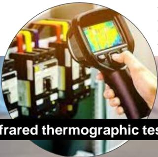
**Infrared thermographic testing**
