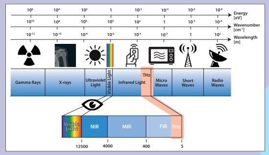
Terahertz radiation is therefore a powerful tool for material characterisation. It can detect features on the meso-scale and reveal material properties, such as characteristic vibrational modes (phonons), permittivity, conductivity and porosity. Measurements are non-contact, avoiding damage and contamination, and allowing stand-off detection.
